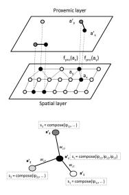
It is possible to build a weighted undirected graph on the proxemic layer. We want to add an edge between two agents when they are close and the perceive each other in a different way. The weight of the edge should be bigger when the two perceptions are very different.
